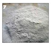
In the slaked lime Ca(OH)2, CaO represents three quarters of the weight, ie more than 75%. It has a small fraction of minerals that gives it a slight runoff (belite). This is a good quality lime which gives a rich mortar, smooth and sticky. It has 5% 2CaO.SIO2, or belite «C2S».
